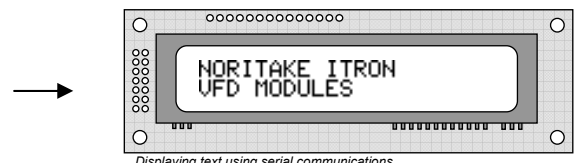
Displaying text using serial communications.
