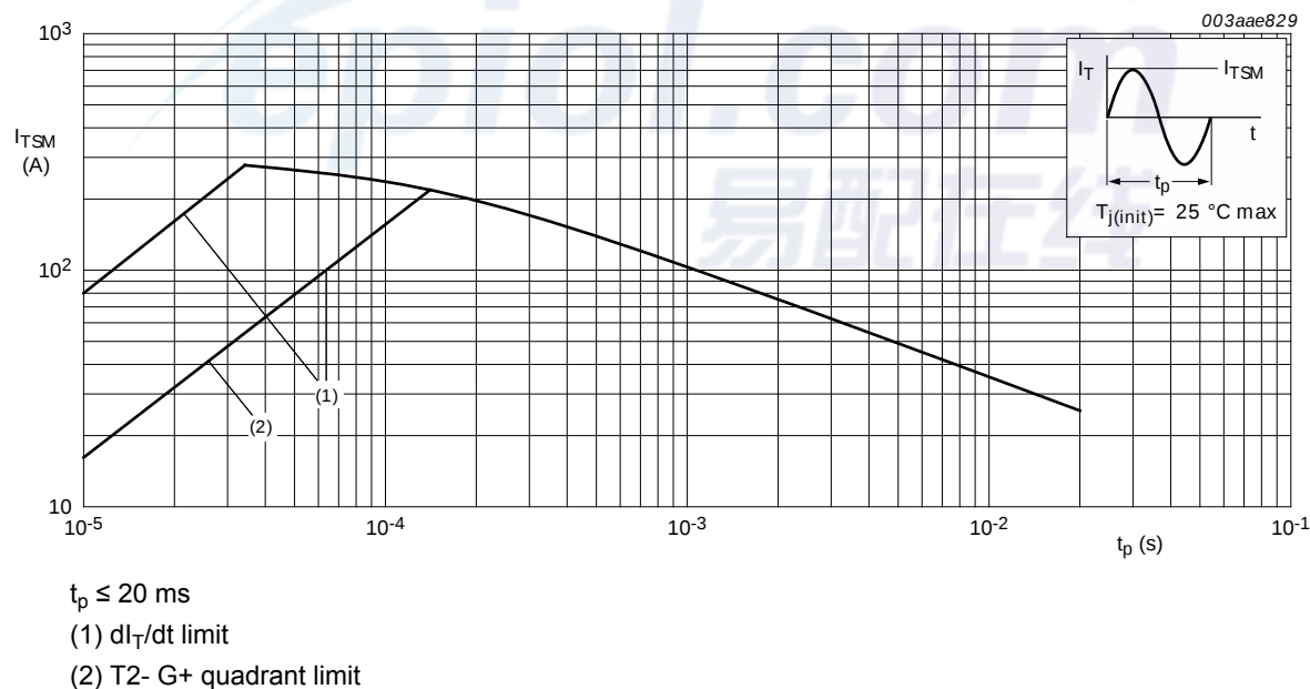
Fig. 5. Non-repetitive peak on-state current as a function of pulse width; maximum values
